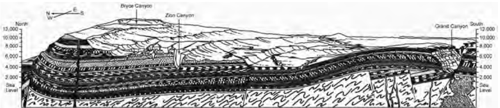
Figure 3. Cross-section through the Grand Canyon-Grand Staircase region showing the extent of the rock layers
