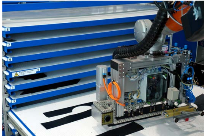
Figure 5: Automated picking process out of a drawer storage unit
