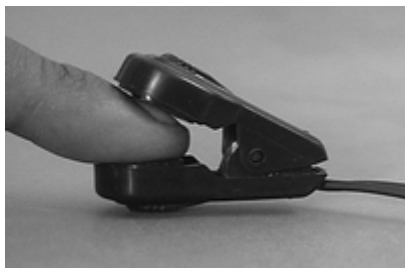
Figure 2. Infrared transmitter and received sensor pair clipped to the finger
