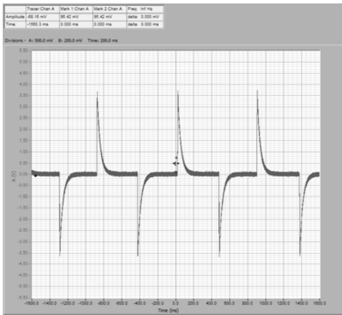
Figure 5. Output response of the amplifier and filter circuit (obtained by connecting a PC based oscilloscope to the circuit)
