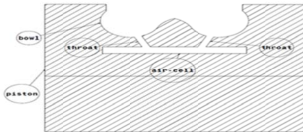
Fig. 2. Schematic view of modify piston
