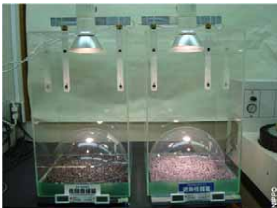
Figure 20 – Laboratory tests on atmospheric temperatures(left: conventional, right:S.H.P.)
