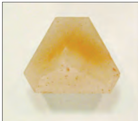
FIGURE 10—Trigonal prism form of Pecos diamonds from Locality 1. Note the color zonation in the upper portion of the crystal. Maximum dimension is 2.2 cm.
