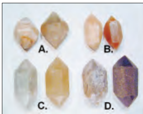
FIGURE 3—Color changes in Pecos valley diamonds after heating at 450°C. All samples illustrated as pairs with the heated sample on the left. Sample pairs A and B from Locality 2, C from Locality 12, and D from Locality 11. The upper left sample is 1 cm long.
