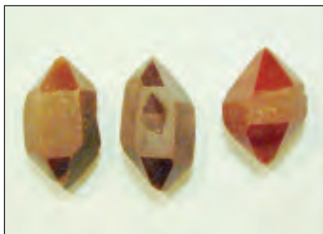
FIGURE 5—Prismatic forms of Pecos diamonds showing rough prism faces ( m ) and smooth rhombohedron faces ( r and z ), even on secondary growths. Note the left and center crystals also show rough ( z ) faces. In contrast, both ( r ) and ( z ) rhombohedron faces on the crystal on the right are smooth. Quartz crystals illustrated are from Locality 11. The left crystal is 1.7 cm long.
