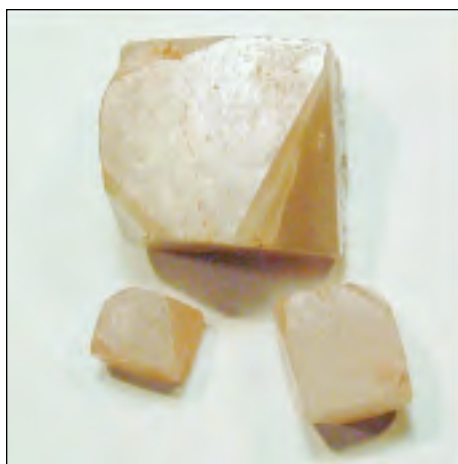
FIGURE 8—Equant pseudocubic quartz crystals from Locality 13, placed at various orientations. The large crystal on the top is 2.5 cm across.
